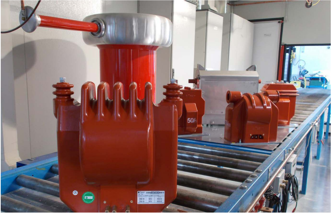
Instrument Transformers at Laboratory
